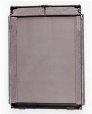
Fig. 3: Frame including PGS foil and PCM inlays
